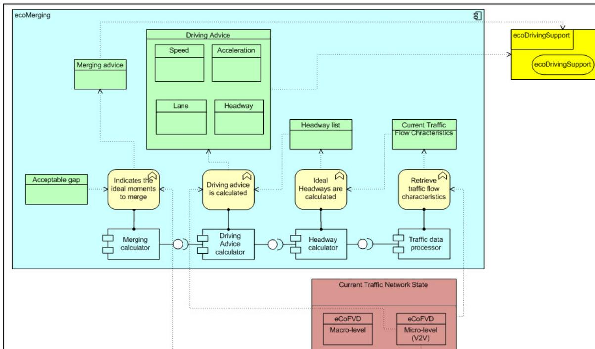
Figure 6. The Application Layer Diagram for Support Merging.
