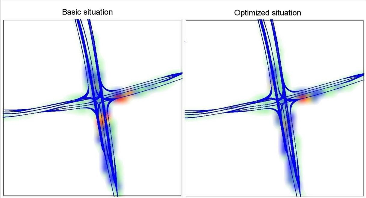
Figure 3. The EnViVer graphical output shows the CO<sub>2</sub> emission in the basic and the optimized situation. Red indicates CO<sub>2</sub> hot spots.
