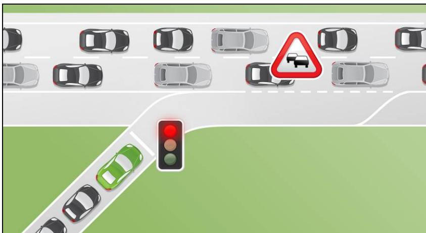
Figure 1. On-ramp with Ramp Metering installation.
