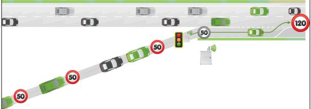
Figure 2. On-ramp with a cooperative Ramp Metering installation. The green cars are also cooperative.
