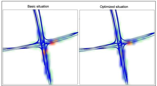
Figure 3. The EnViVer graphical output shows the CO2 emission in the basic and the optimized situation. Red indicates CO2 hot spots.
